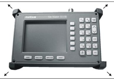
Figure 4-1. Removing the Corner Bumpers
