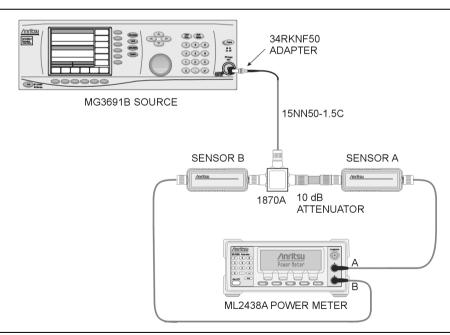
Figure 2-4. Power Meter Verification Pre-test Setup
