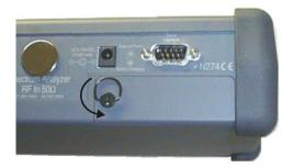
Figure 3-2. Rotate the Battery Access Door Handle
