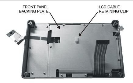
Figure 4-4. Front Panel Backing Plate
