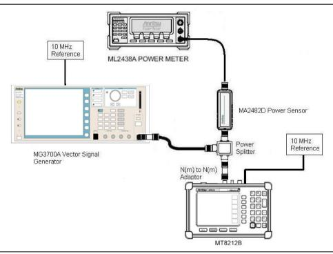
Figure 2-8. GSM RF Measurement Test Setup
