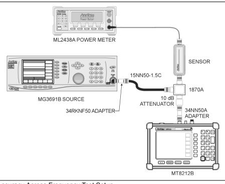
Figure 2-2. Level Accuracy Across Frequency Test Setup
