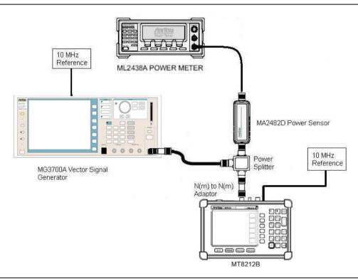
Figure 2-10. iDEN Signal Analyzer Setup
