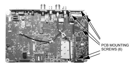
Figure 4-10. T1/E1 Tester PCB
