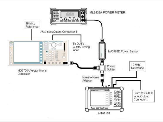
Figure 2-7. EVDO Signal Analyzer Option Verification
