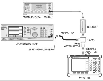
Figure 2-5. Power Meter Verification Setup
