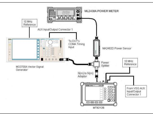
Figure 2-9. CDMA Signal Analyzer Setup
