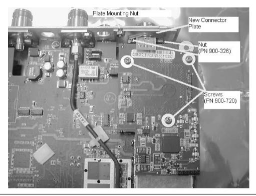
Figure 4-9. Power Monitor PCB Assembly Replacement
