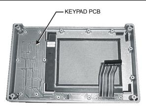
Figure 4-5. Front Panel Keypad PCB Location
