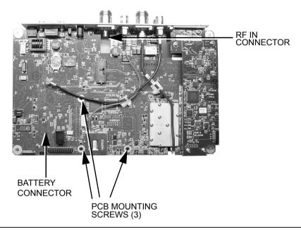
Figure 4-7. Main PCB (shown with T1/E1 PCB installed)
