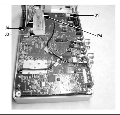
Figure 4-2. Cell Master Front Panel Cable Connections
