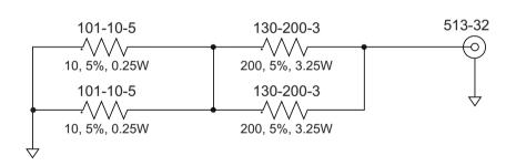
Figure B-2. Anritsu Model T3377 Low Current Test Fixture (for Option 10 and 10A)
