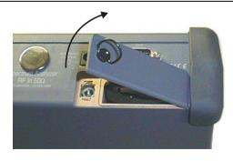
Figure 3-3. Removing the Battery Access Door
