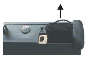
Figure 3-4. Removing the Battery
