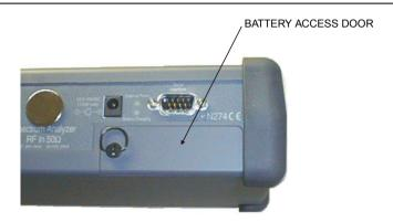
Figure 3-1. Battery Access Door Location
