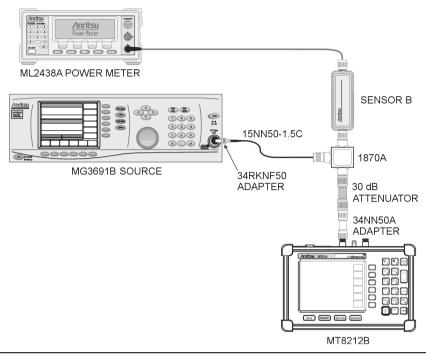
Figure 2-3. Level Accuracy Test through Power Setup
