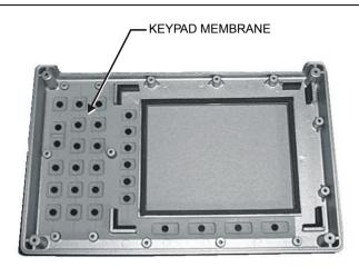
Figure 4-6. Front Panel Keypad Membrane
