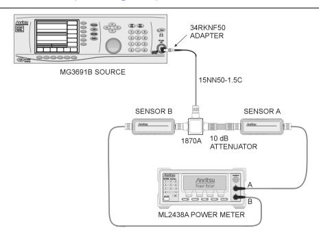
Figure 2-1. Level Accuracy Across Frequency Test Pre-test Setup
